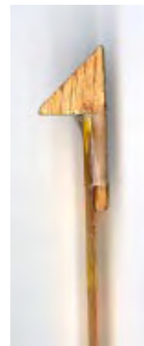
For wing-chords. Cheap plastic ruler & piece of wood taped on for a carpal stop
